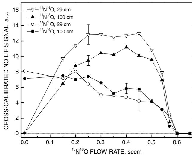
Fig. 6 LIF signal intensities for  $^{14}\text{N}^{18}\text{O}$  and  $^{14}\text{N}^{16}\text{O}$  as functions of the  $^{15}\text{N}^{18}\text{O}$  titration flow rate at 1200 K. The plotted values represent integrated photon counts for several selected lines, as indicated in Fig. 5. The estimated uncertainties (indicated by the error bars) are shown for only one data point in each curve, for clarity.
