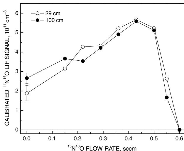
**Fig. 4** LIF signal intensity for  $^{14}\text{N}^{16}\text{O}$  as a function of the  $^{15}\text{N}^{16}\text{O}$  titration flow rate at 1200 K. The plotted values represent integrated photon counts for several selected lines, as indicated in Fig. 3. The error bars are estimated uncertainties, and they are shown for only one data point in each curve, for clarity.
