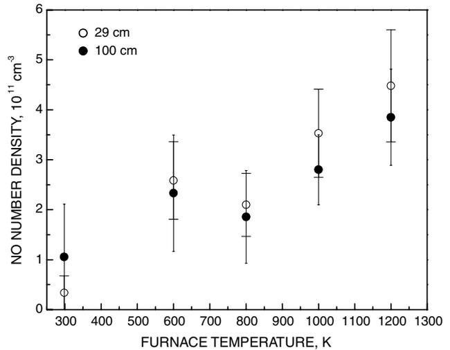
Fig. 7 Number density of surface-produced  $^{14}\text{N}^{16}\text{O}$  as a function of temperature for two positions down the diffusion tube. The data were obtained using  $^{15}\text{N}^{16}\text{O}$  titration, with a titration flow rate corresponding to 70% of the endpoint. The background signal was subtracted to obtain the  $^{14}\text{N}^{16}\text{O}$  density due solely to the O atoms introduced by titration (see text).
