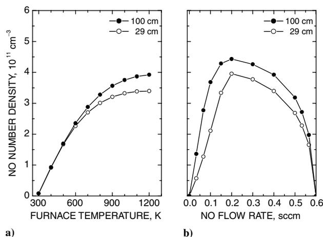
**Fig. 8** The number density of surface-produced NO at distances of 29 and 100 cm from the sidearm opening as a) a function of furnace temperature for a titration gas flow of 0.4 sccm, and b) a function of titration gas flow at a furnace temperature of 1200 K.
